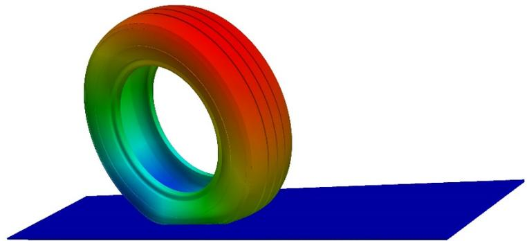
*Fig. 1: Simulating contact of rolling tire and roadway surface.*
