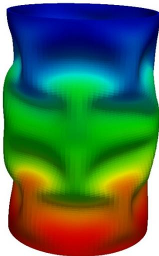
**Fig. 3:** Example for self-contact: bulging can.
