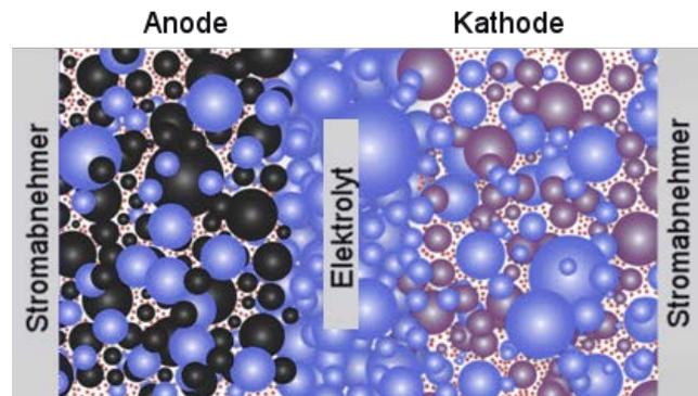
**Abb. 2:** Exemplary solid-state cell with composite anode.
